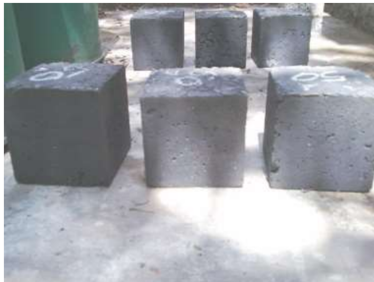
Geopolymer concrete cubes (G50)
