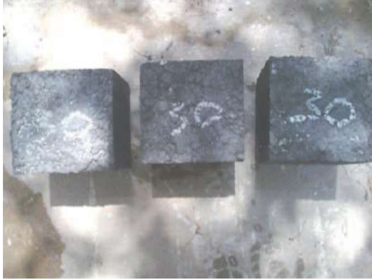
Geopolymer concrete cubes (G30)
